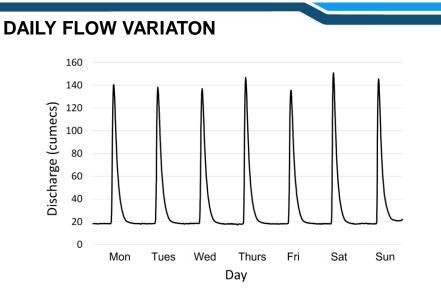
Discharge recorded from Vanderkloof Dam at gauging station (station D3R003) over a one-week period (01/01/2020 - 08/01/2020). Pattern shows the daily hydropeaking resulting from hydroelectric power generation releases.
